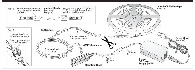
Tresco Lighting's LED FlexTape light system is designed to adhere to a smooth, clean surface (indoor locations only). To be used with Tresco DC Power Supplies Only.
